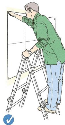
Good practice 2 clear rungs Do not work any higher up this type of steps
